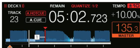
When the set point is reached, the loop is set automatically and loop playback begins.
