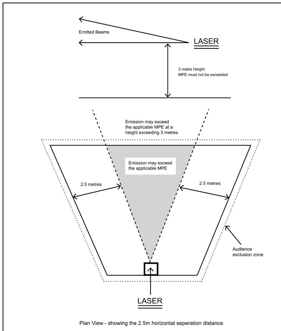
**Note.** The 3 metre height specified is not the height of the actual laser unit, but it refers to the height of the laser beams emitted.
